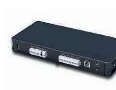
GAT NET.Controller M 7020 Master Controller
